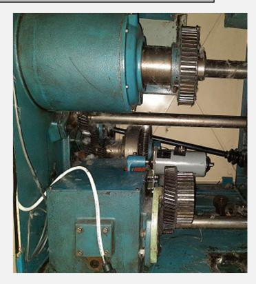
MODIFIED DRIVE SYSTEM FOR BOBBIN & RAIL
